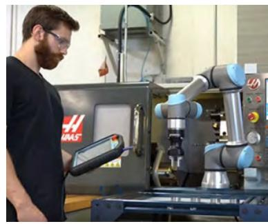
involving multiple machines and inspection equipment each part will have a program for each machine included along with the robot. Each changeover requires synchronized program loading so the robot and all associated machines get the correct program for the part that will be processed.
